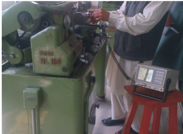
Figure 2 : Experimentation and readings with vibration meter
